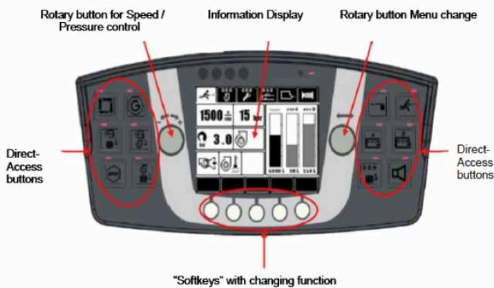
Figure 02: Control elements at the HMI control unit
