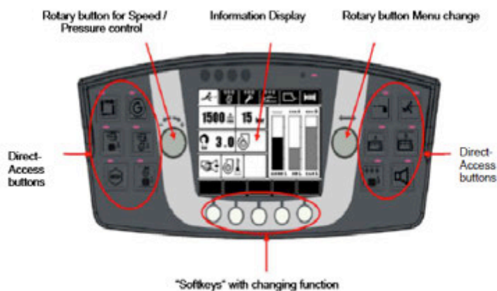
Figure 02: Control elements at the HMI control unit
